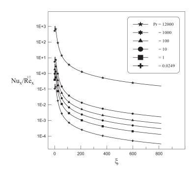
Figure 17. Effect of Prandtl number on Nusselt number distribution: Re = 100 (parabolic surface), Da =  $2 \times 10^7$ ,  $\Lambda = 0.4$ , VR = 1
