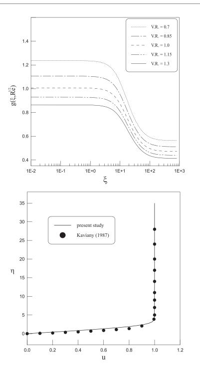
Figure 12. Local velocity profile: Re = 0 (flat plate), Da =  $2 \times 10^7$ ,  $\Lambda = 0.4$
