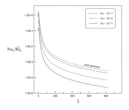
Figure 18. Effect of Darcy number on Nusselt number distribution: Pr = 1,  $\Lambda = 0.4$ , Re = 100(parabolic surface), VR = 1
