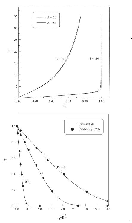
Figure 14. The effect of inertia parameter ( $\Lambda$ ) on local velocity distribution: Da = 2 × 10<sup>7</sup>, Re = 100, VR = 1
